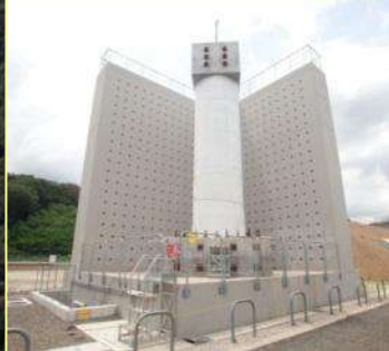
Tri-axial loading system for structures
